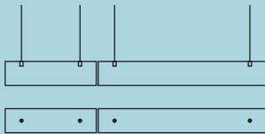
*As a rule, if the suspended luminaire consists of multiple lengths, it is required to install two suspension cables per each cut section.*
