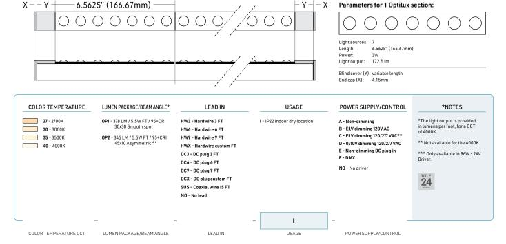
Parameters for 1 Optilux section:
