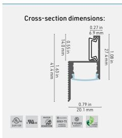
A cove without a cove. Go beyond the traditional idea of a 6"x6" or 9"x9" box to create a cove light. The 1540 profile allows you to create a cove detail with only a depth of  $3\!\!4$  of an inch. This mud-in aluminum channel fits with both  $5\!\!4$ -inch and  $1\!\!2$ -inch drywall with the help of a simple clip that snaps into place. This lighting solution creates ceiling coves, wall coves, mid-wall applications, tray ceiling lighting, and highlights around and into corners.
