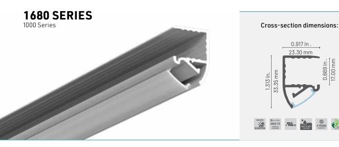
Here is an aluminum LED profile which is installed simply by sliding it over a standard 5%" shelf. This snap on profile with a variety of snap on lenses results in a very fast and easy installation. Shining light downward at a 35 degree angle, the objects under the shelf are beautifully illuminated.
