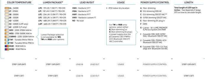
\*NOTE: The light output is provided in lumens per foot, for a CCT of 4200K and no lens. Please refer to the optics page for CCT and translucency conversion factors. \*\* Only available in 96W - 24V Driver
