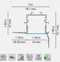
The 8540 Pro profile is designed to disappear into the structure, merging the light source with the surface. Its  $90^{\circ}$  edge on one side makes it ideal for contour lighting application. Very versatile with 15 LED light sources to choose from 2400 K to 6200 K including WarmDim, Tunable White, RGB and RGB white. Its refined look harmonizes perfectly with any project.
