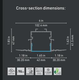
The 8550 Pro profile is designed to disappear into the structure, merging the light source with the surface. Very versatile with 15 LED light sources to choose from 2400 K to 6200 K including WarmDim, Tunable White, RGB and RGB white. Its refined look harmonizes perfectly with any project.
