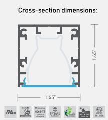
The 8800 Luxline is an aluminum channel designed for long and bold linear lines of light. It is integrated with our energy-efficient Luxline 120-volt LED technology for a custom linear lighting solution. The 8800 Luxline can be suspended, surface mounted, or recessed, permitting a vast number of applications. Attain a refined look without any pixelation that will harmonize perfectly in any space when seeking long linear runs of light.
