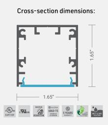
The 8800 is an aluminum channel designed to provide a bold linear line of light. Select from a wide array of optics, light outputs, and LED options to meet the needs of your project. This aluminum channel can be suspended, surface mounted, or recessed permitting a vast number of applications with this linear lighting solution.
