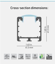
The **9400 profile** with its twin mounting channels allows for a **wide range of installation options**. Whether on swivel arms, on a surface, or suspended, it can be built in complex spatial configurations using **corner joiners**. Its rugged build in 6063-T5 aluminum alloy will withstand abuse in demanding applications and extreme weather, all of it with an understated elegance.
