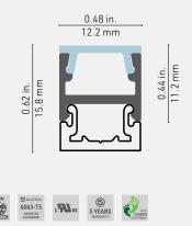
An extremely small aluminum channel that gives you a linear pin of light to create a beautiful modern look. The extra slim channel can be recessed or surface mounted for the desired effect. This profile is easily installed with a specially designed bracket that snaps into place.
